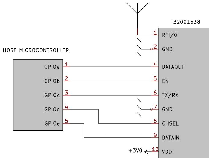
In this mode, control pins on microcontroller side, must be configured as follow:
