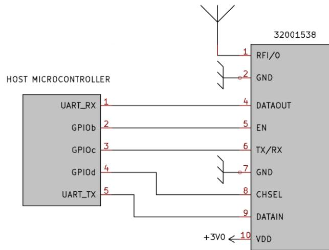
In this mode the control pins on the microcontroller side must be configured as follow:
