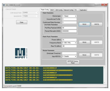
NOTE: to check if a device is connected, verify that each input command has an answer in the petrol green box below.
