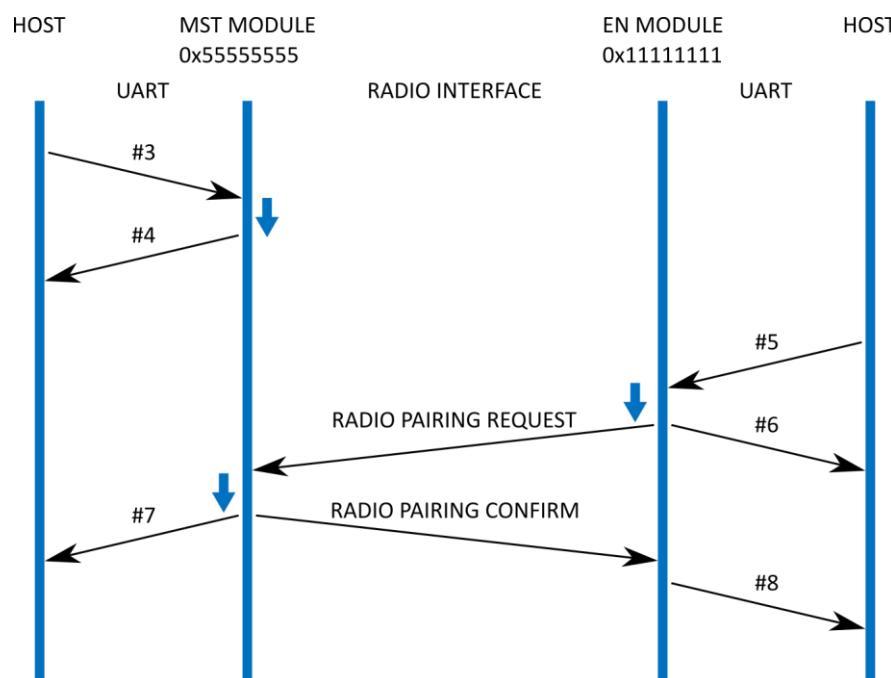
When the pairing procedure ends, the pairing mode has to be disabled on MST.
