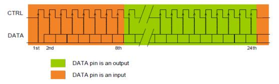
As stated in previous discussion, programming of the configuration register is triggered by a rising edge on the CTRL line while TX DATA line is held low. Upon detection of such condition, the data applied to the TX DATA pin is accepted as register configuration information, the data bits are clocked on subsequent rising edges of the clocking signal applied to the CTRL pin. Note that, once triggered, all 24 clock cycle must be issued to the 32001372 TX module.
