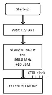
At power up the 32001372 TX module waits T\_START time to elapse and then automatically starts in NORMAL MODE with FSK modulation at 868.3MHz. It can work indefinitely in NORMAL MODE or it can switch to EXTENDED MODE.
