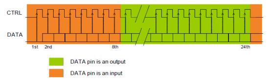
As stated in previous discussion, programming of the configuration register is triggered by a rising edge on the CTRL line while TX DATA line is held low. Upon detection of such condition, the data applied to the TX DATA pin is accepted as register configuration information, the data bits are clocked on subsequent rising edges of the clocking signal applied to the CTRL pin. Note that, once triggered, all 24 clock cycle must be issued to the 32001371 TX module.
