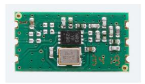
32001371 TX module is an SMD 433.92MHz OOK-FSK transmitter. It can operate in:
