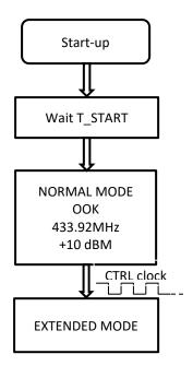
At power up the 32001371 TX module waits T\_START time to elapse and then automatically starts in NORMAL MODE with OOK modulation at 433.92MHz. It can work indefinitely in NORMAL MODE or it can switch to EXTENDED MODE.
